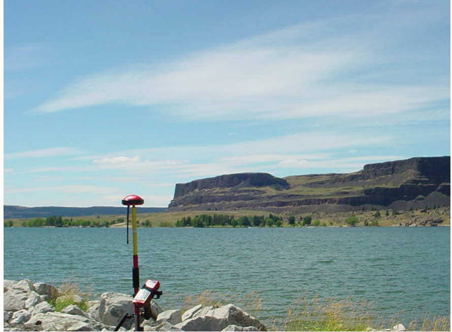
Longer baselines: this site near Steamboat Rock in central Washington is 50 kilometers from each of the adjacent RTN reference stations; consistent and reliable corrections available on-demand 24/7
